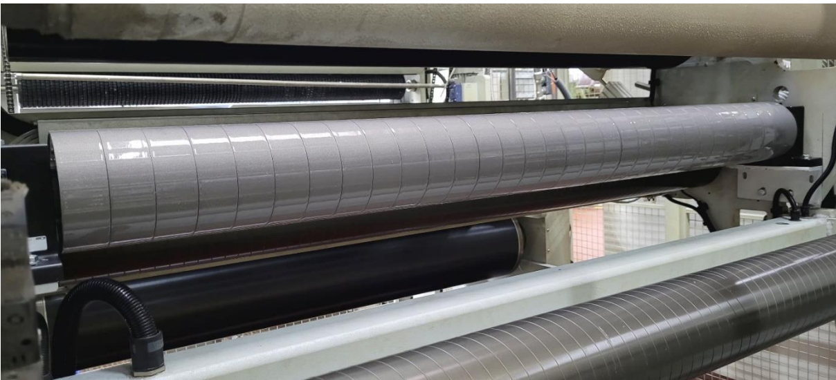
Illustration 1: The FMS-segFORCE features up to 50 independent force sensors that measure the smallest tension deviations between the segments. It is particularly suitable for processing elastic and sensitive materials.
