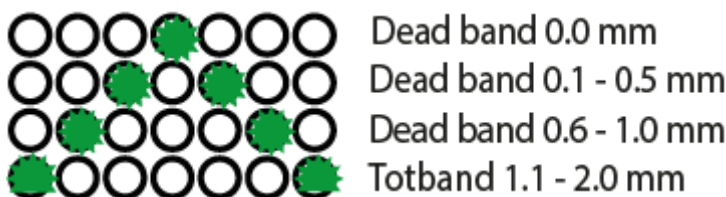
Fig 9: LED indication of Dead Band values BKS015_BA_Manual.ai
