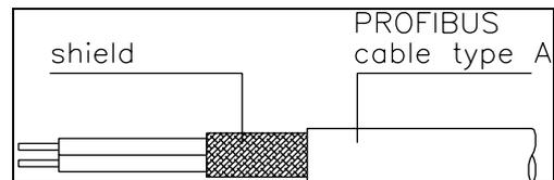
**fig. 7: Preparation of the PROFIBUS cables**
