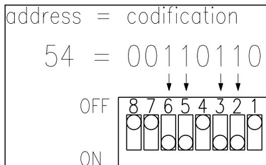
**fig. 10: Codification of the PROFIBUS address (Example with address 54)**
