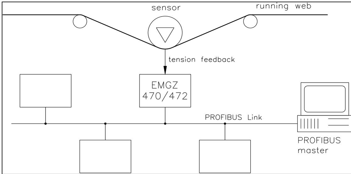
fig. 1: Basic structure EMGZ470A.W/472A.W Tension Measuring Amplifier E470001e
