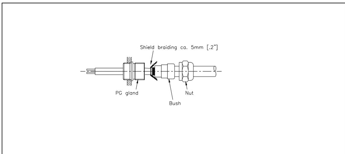
fig 6: Connecting the shield
