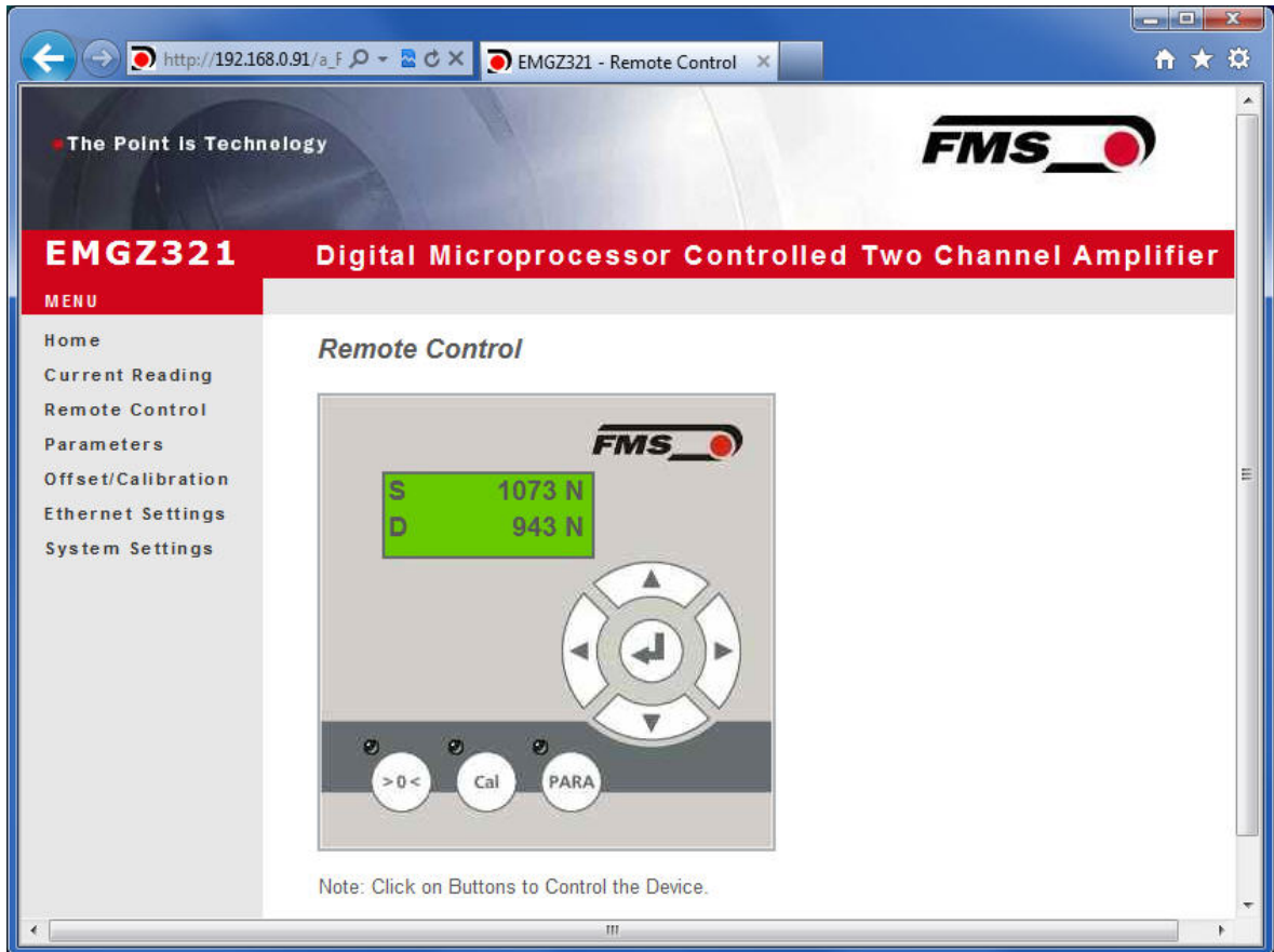
Fig. 31: Remote Control Screen to operate the EMGZ321 via Ethernet Remote Cont
