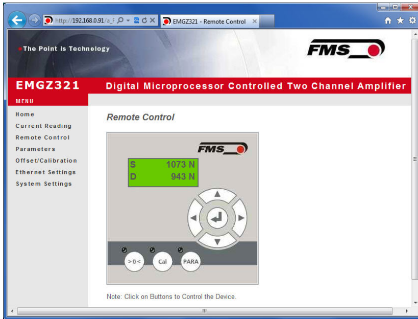
Fig. 25: Remote Control Screen to operate the EMGZ321 via Ethernet Remote Cont
