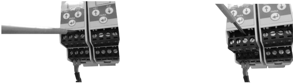
Figure 4: Detachable terminal blocks: use a small slotted screwdriver as a lever
