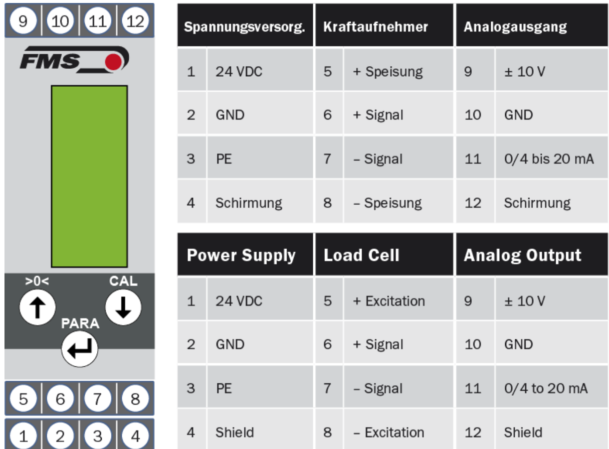
Figure 3: electrical connections
